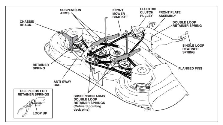
Position front plate assembly between front mower brackets. Raise deck and plate assembly to align holes and insert flanged pins. Secure pins with double loop retainer springs between the plate and mower brackets.
